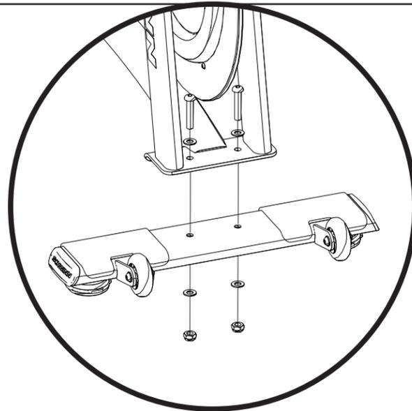
**STEP 1:** Install the front stabilizer using a 5mm allen key and a 17mm open-ended wrench to secure two (2) pieces each of the M10 x 50mm screws and M10 nuts. Be sure to place one (1) piece of the M10 washer between the nuts and the stabilizer as well as the screws and the frame. **Repeat this step to attach the rear stabilizer to the frame.**
