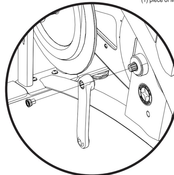
**STEP 6:** IF 4III POWER SENSOR IS BEING INSTALLED, SKIP THIS STEP AND REFER TO INSTALL DOCUMENTATION FOR THE 4III CRANK ARM. Install the left crank arm onto the left side of the bottom bracket ensuring that the right crank arm is at the 12 o'clock position while the left crank arm is at the 6 o'clock position. Finally, use a torque wrench and a 8mm allen key socket to secure one (1) piece of the crank bolt through the crank arm and into the bottom bracket, torquing to 33-37 ft-lbs (48 Nm)
