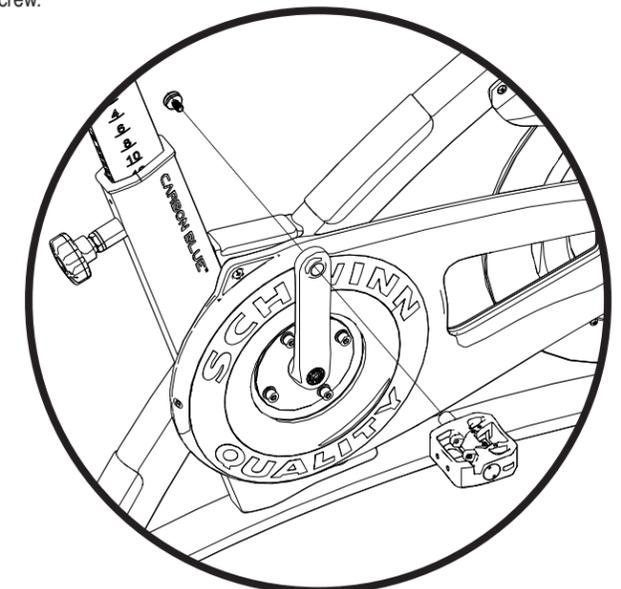
**STEP 7:** Insert the right pedal into the rider right side crank arm and tap firmly with a rubber mallet. Finally, use a torque wrench and a 8mm allen key socket to secure one (1) piece of the crank bolt from the other side of the pedal, torquing to 33-37 ft-lbs (48 Nm). **Repeat this step for the rider left side pedal.**
