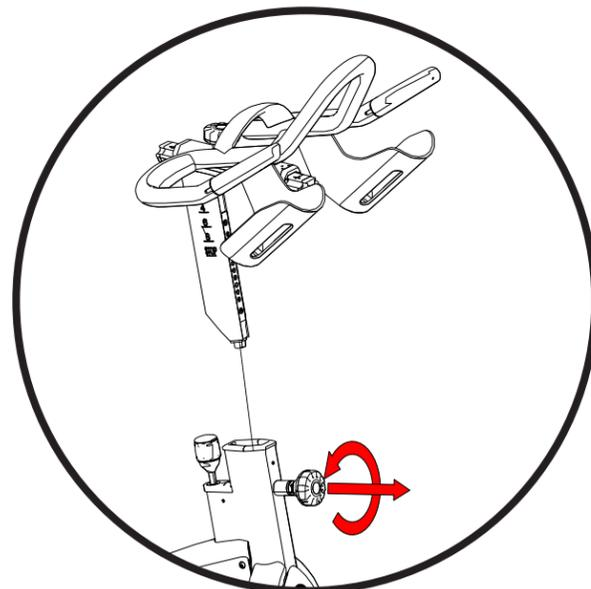
**STEP 5:** Slide the handlebar post assembly built in Step 3 into the frame by loosening the height adjustment pop pin, then pulling outwards on the pin while sliding the handlebar post assembly into the frame.
