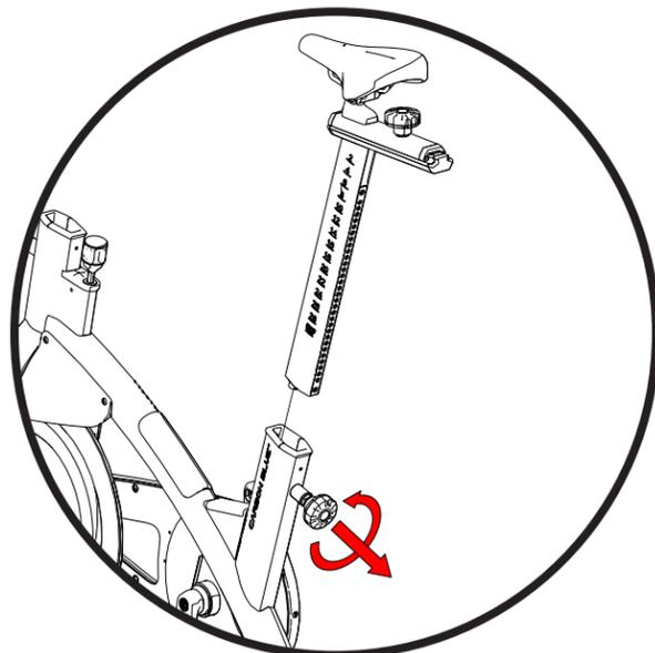
**STEP 4:** Slide the seat post assembly built in Step 2 into the frame by loosening the height adjustment pop pin, then pulling outwards on the pin while sliding the seat post assembly into the frame.
